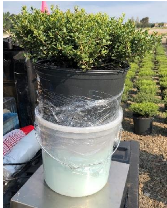
Figure 2: "Skirted" sample for irrigation efficiency analysis
